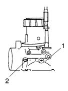
The following variations apply to air screw (2) adjustment for 2-cycle engines:
